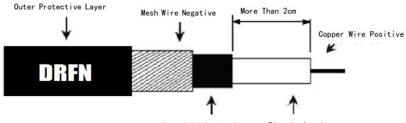
Signal Isolation Layer Plastic Insulator
